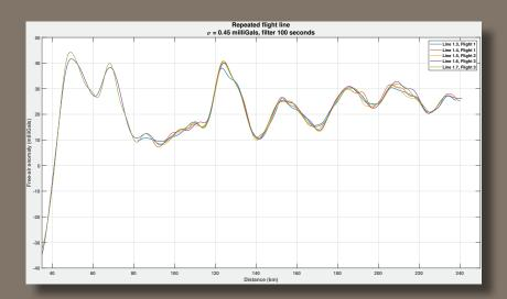
The TAGS-7 data shown above are five repeat measurements of the free-air anomaly acquired on a flight line at 3120 meters altitude. The terrain was generally mountainous, ranging from 1450 to 2900 meters above sea level. With a 100 second filter, the standard deviation of the repeats was 0.45 mGals.
