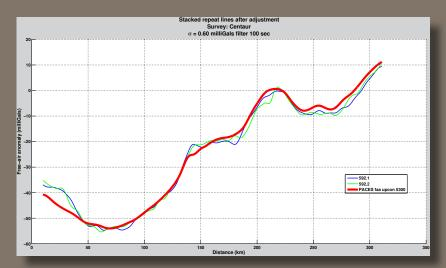
The TAGS-7 data shown above are two repeat measurements of the free-air anomaly acquired on a flight line at 5460 meters altitude. The red line is the free-air anomaly derived from public-domain land gravity data, upward continued to the flight height. The terrain was varied, ranging from 60 to 650 meters above sea level. With a 100 second filter, the standard deviation of the repeats was 0.60 mGals
