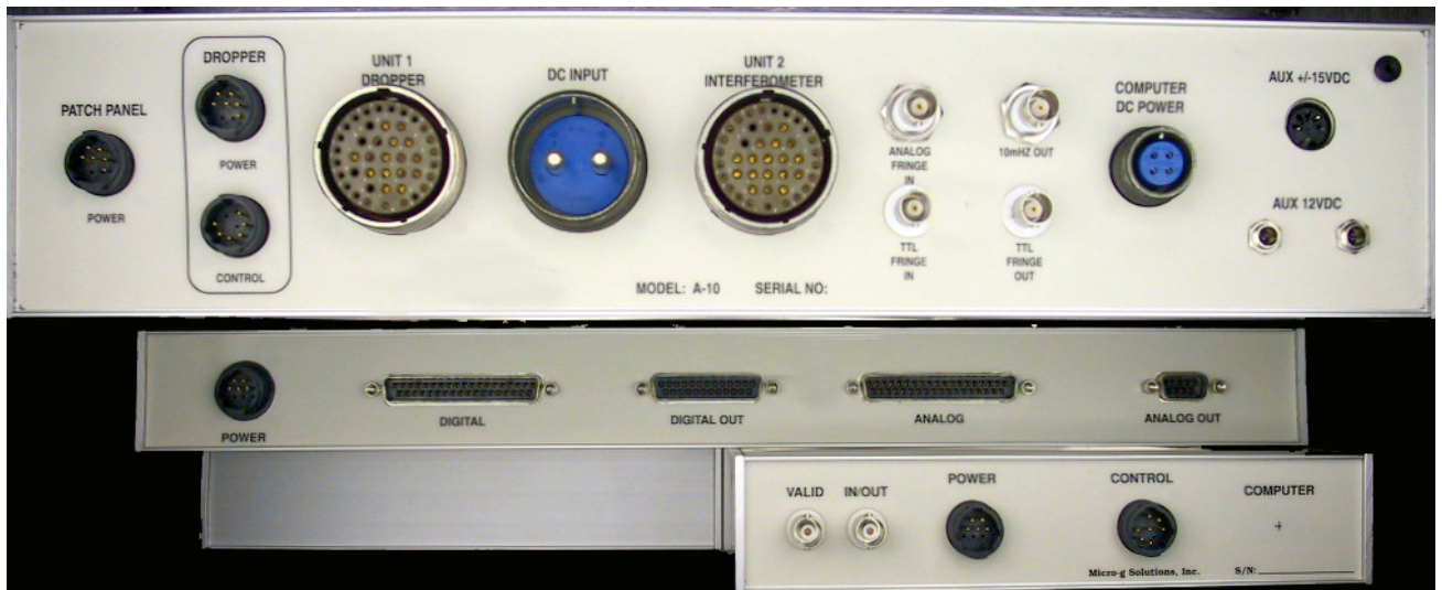
Figure 5. Electronics Rack, rear view. Top to bottom: Control Panel, Patch Panel, Dropper Controller.
