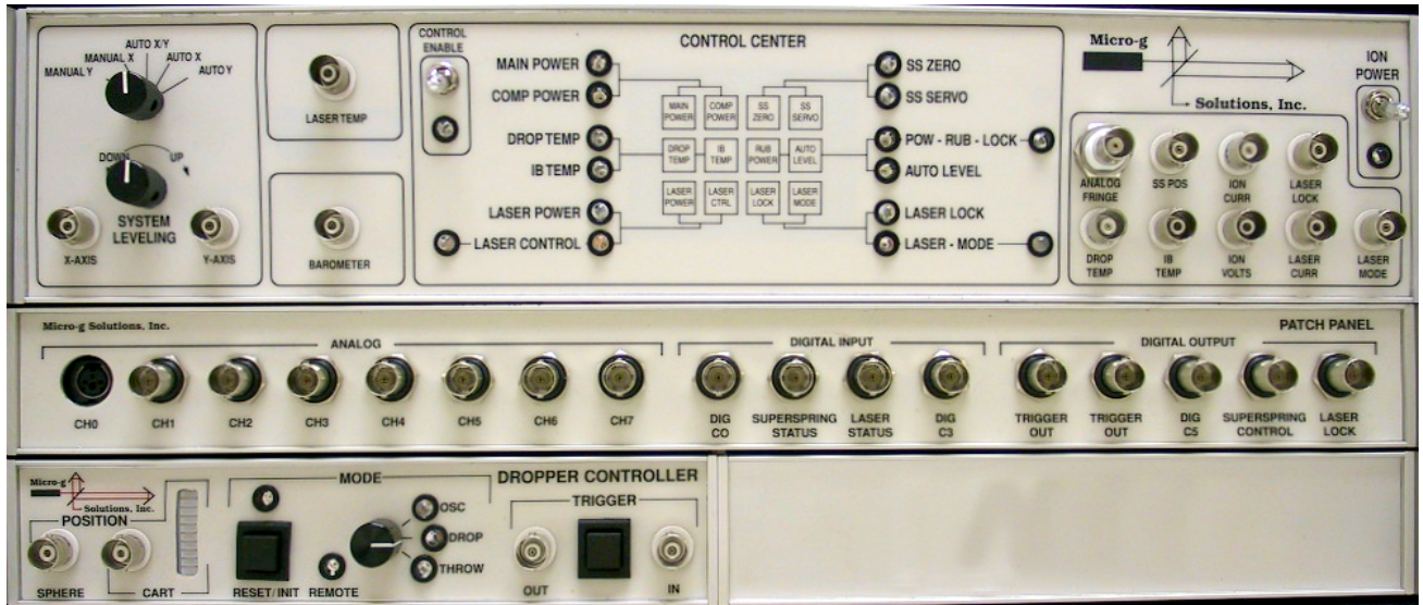
Figure 4. Electronics Rack, front view. Top to bottom: Control Panel, Patch Panel, Dropper Controller.
