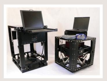
Shown above are the original TAGS on the left (without safety cages installed), and TAGS-7 on the right (no safety cages necessary).
