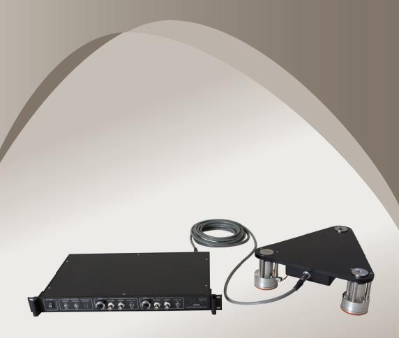
A precision leveling and stabilizing platform for gPhone, gPhoneX and other instrumentation
