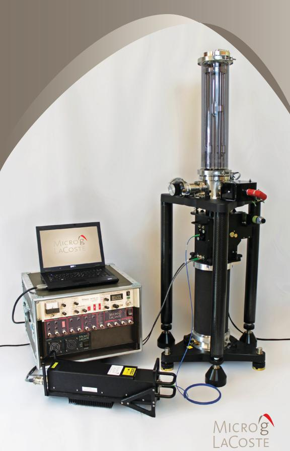
ince its introduction in 1995, the FG5 has become the industry standard in absolute gravity instrumentation, and now Micro-g LaCoste is proud to produce the latest version: the FG5-X. Based directly on international standards of time and distance, the FG5-X provides unparalleled accuracy and precision. Whether applied in geophysical research, environmental monitoring, or laboratory metrology, the FG5-X is still the highest quality, most versatile absolute gravimeter available today.
