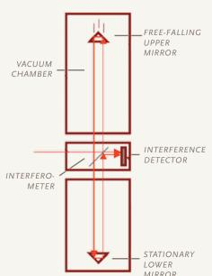
proclaimed the ballistic free-fall method as an official primary method for measuring gravity.
