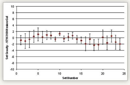
Shown above are the results of a 24-hour site occupation (24 sets of 100 drops each). The set scatter is on the order of 1 µGal, indicating sub-µGal measurement precision.
