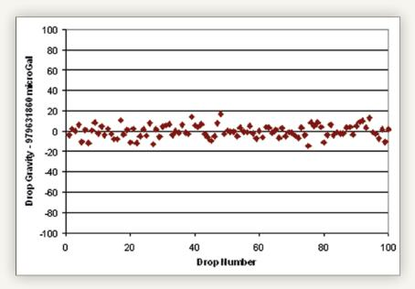
Shown above are individual measurements in a laboratory setting. The standard deviation between drops is better than 6  $\mu$ Gal. Note that the measured absolute gravity value, in this case 979 631 858  $\mu$ Gal, is computed and reported in real time.
